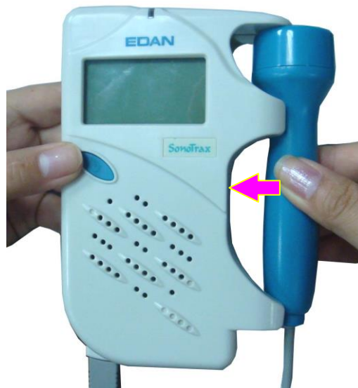
Figure 3-5 Placing the probe
